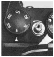
speeds one is recommended to use a cable release which can be screwed into the release button thread. In so doing the camera should be mounted on a tripod.
